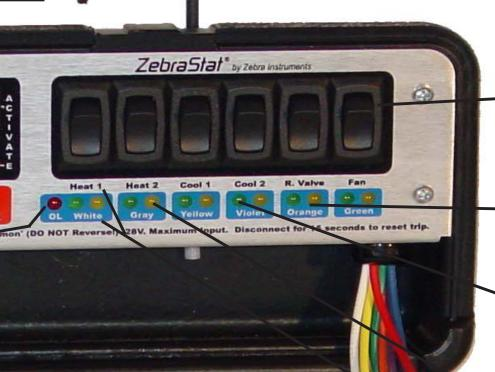
Quick Operating Instructions (tul version in ma has 3 operating modes, plus Voltage Check and Circuit Protection
