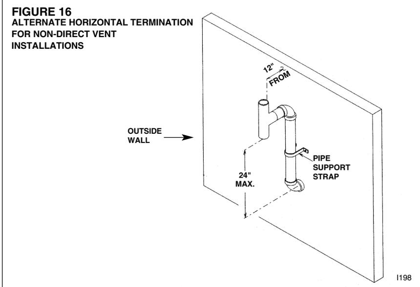
“rub-a-tex” insulation may also be used as long as there is no heat tape applied to the vent pipe. For horizontal runs where water may collect, wrap the vent pipe with self-regulating 3 or 5 watt heat tape. The heat tape must be U.L. listed and installed per the manufacturer’s instructions.
