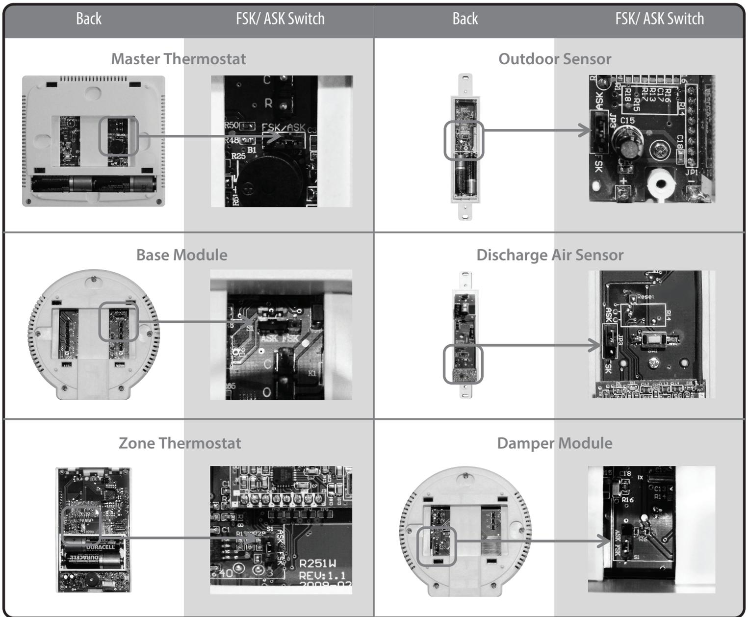
**NOTE:** Anytime a jumper pin switch has been changed, the device needs to be reset or power cycled to configure the changed setting
