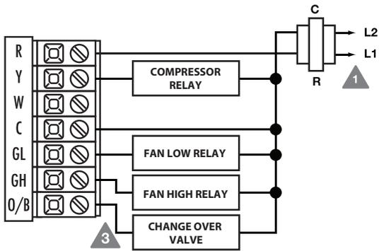
**Typical 2H/1C Heat Pump system: 2 speed fan**
