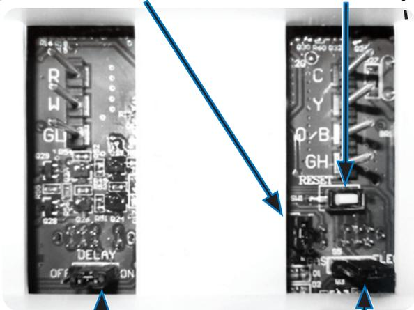
Select delay **ON** or **OFF** with the jumper pin
