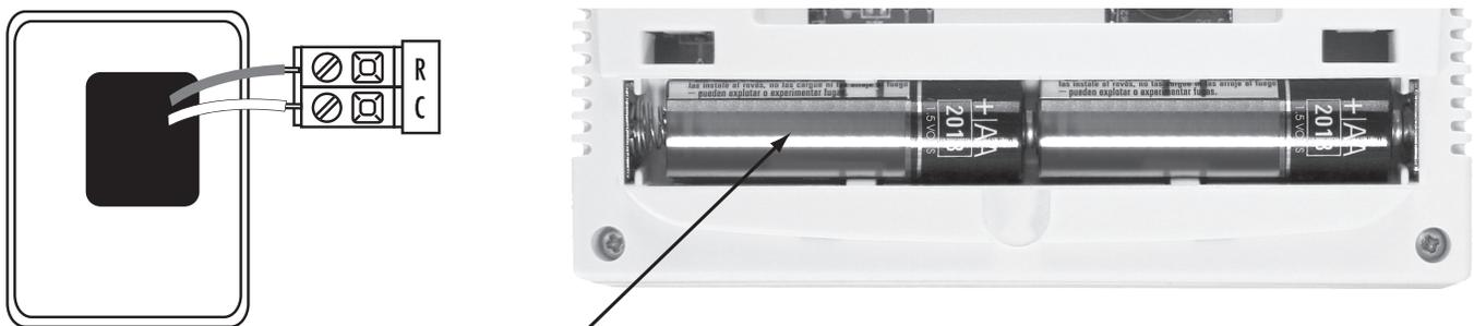
Insert 2 AA Alkaline batteries (included).
