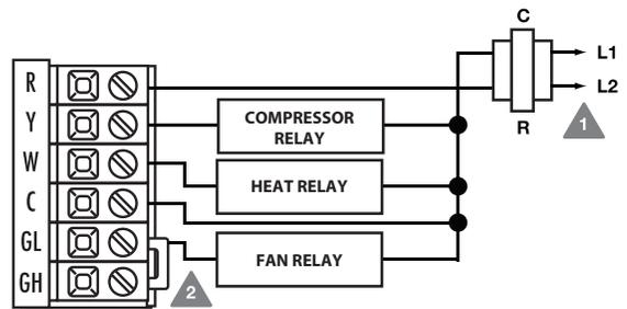
**Typical 1H/1C Heat Pump system: 2 speed fan**
