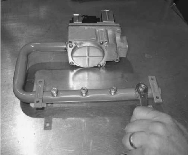
7. Replace the orifices with the proper high-altitude orifices. Screw them in hand tight and secure in place (with the wrench or socket) 1/4 turn from hand tight.
