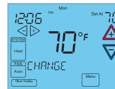
**Air Filter Maintenance** - When the system has run for the selected length of time, the scrolling message area will show “**CHANGE FILTER**”
