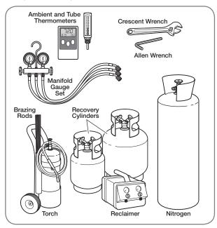
**ACAUTION:** R-410A systems operate at higher pressures than R-22 systems. Do not use R-22 service equipment or components on R-410A equipment.
