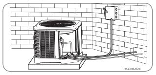
The vapor line must be insulated for its entire length to prevent dripping (sweating) and prevent performance losses. Closed-cell foam insulation such as Armaflex and Rubatex® are satisfactory insulations for this purpose. Use 1/2" [12.7 mm] minimum insulation thickness. Additional insulation may be required for long runs.
