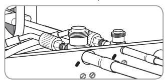
At this time gauges must be connected to the access fitting on the liquid line (small) service valve and the common suction port connected to the common suction line between the reversing valve and compressor to check and adjust charge.
