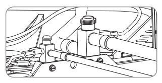
Gauges must be connected at this point to check and adjust charge. Do not replace caps yet.
