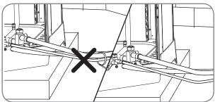
Do not allow the vapor line and liquid line to be in contact with each other. This causes an undesirable heat transfer resulting in capacity loss and increased power consumption.
