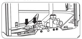
Remove the caps and Schrader cores from the pressure ports to protect seals from heat damage.
