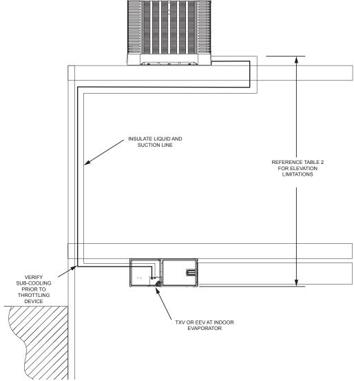
For applications that are considered to have a long line set with the outdoor unit above the indoor unit the following is required:
