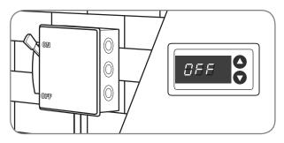
At initial start-up or after extended shutdown periods, make sure the crankcase heater is energized for at least 12 hours before the compressor is started. (Disconnect switch is on and wall thermostat is off.)
