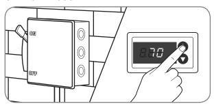
With thermostat in the "Off" position, turn on the power to the furnace or air handler and the heat pump. Start the heat pump and the furnace or air handler with the thermostat. Verify that the outdoor unit is operating in second stage and the indoor air mover is delivering the correct airflow for the system size.
