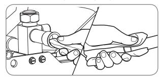
Clean the inside of the fittings and outside of the tubing with a clean, dry cloth before soldering.
