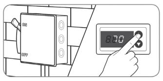
With thermostat in the "Off" position, turn the power on to the furnace or air handler and the heat pump. Start the heat pump and the furnace or air handler with the thermostat. Verify that the outdoor unit is operating in second stage and the indoor air mover is delivering the second-stage airflow for the system size.
