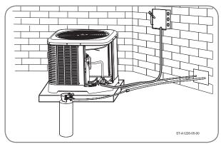
Blow out the liquid and vapor lines with dry nitrogen before connecting to the outdoor unit and indoor coil. Any debris in the line set will end up plugging the expansion device.
