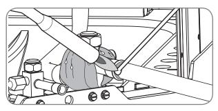
Braze the tubing between the outdoor unit and indoor coil. Flow dry nitrogen into a pressure port and through the tubing while brazing, but do not allow pressure inside tubing which can result in leaks. Once the system is full of nitrogen, the nitrogen regulator should be turned off to avoid pressuring the system.
