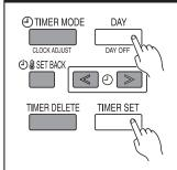
Press the DAY (DAY OFF) button and TIMER SET button simultaneously for 2 seconds or more to activate the part lock function and lock all of the buttons on the remote controller except the START/STOP button, SET TEMP. buttons, MODE button, and FAN button. Press the buttons again for 2 seconds or more to deactivate the part lock function. When the part lock function is activated, the part lock, the **PL** display flashes.
