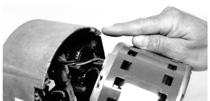
FIGURE 22 MOTOR ALIGNMENT PIN
