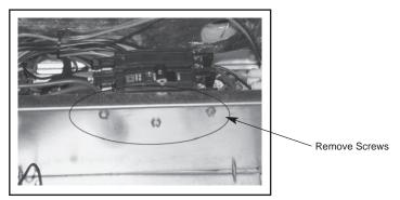
4. Remove capacitor to help prevent damage to the coil. (1/4" Socket)
