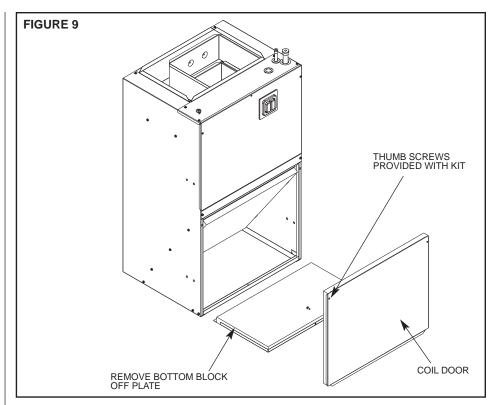
• **Bottom Return Conversion Kit RXHK-** is used to divert the return air from the factory standard front return to a bottom return.
