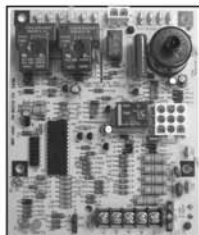
INTEGRATED FURNACE CONTROL
