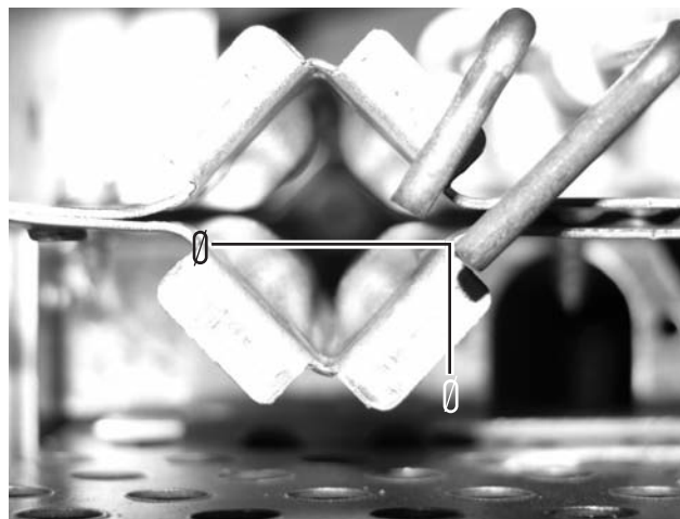
UPFLOW OPTIMUM IGNITOR LOCATION
