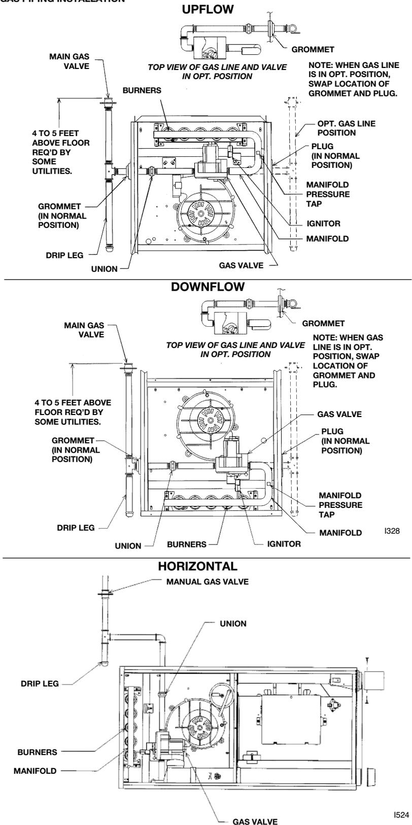
**IMPORTANT:** DO NOT RUN A FLEXIBLE GAS CONNECTOR INSIDE THE UNIT. Extend the 1/2" black pipe from the gas valve to the outside of the cabinet. Connect any flexible gas connector from there to the gas piping.
