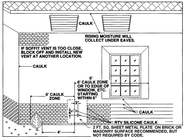
surfaces, unless a rust-resistant sheet metal or plastic backing plate behind vent. See Figure 23.
