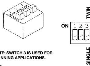
NOTE: SWITCH 3 IS USED FOR TWINNING APPLICATIONS.
