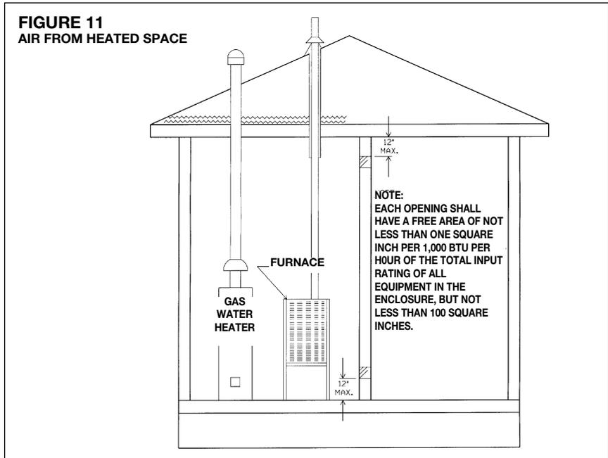
through vertical ducts as shown in Figure 12, each opening shall have a minimum free area of 1 square inch for each 4,000 BTUH of total appliance input rating in the enclosure.
