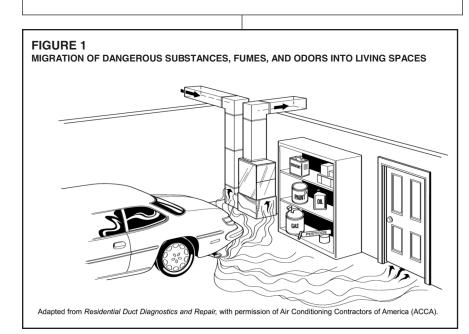
Proper balance and sealing of the duct system improves the efficiency of the heating and air conditioning system and improves the indoor air quality of the home by reducing the amount of airborne pollutants that enter homes from spaces where the ductwork and / or equipment is located. The manufacturer and the U.S. Environmental Protection Agency's Energy Star Program recommend that central duct systems be checked by a qualified contractor for proper balance and sealing.
