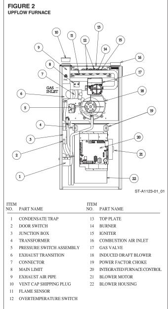
which varies the input rate of the furnace proportionally to the signal from the controller. The modulating furnace can operate anywhere from 40% to 100% of the nameplate input of the furnace.
