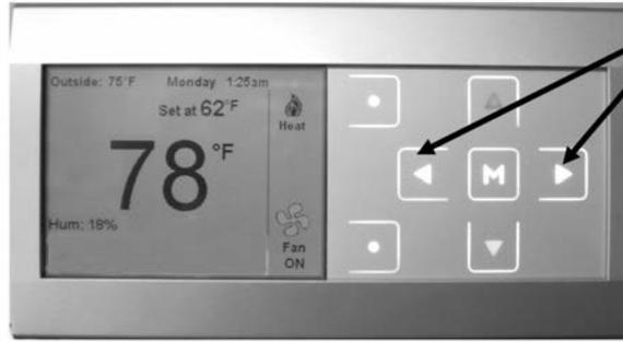
1. From the main screen, press the left and right arrow keys together at the same time for at least 3 seconds. The next screen below will appear.
