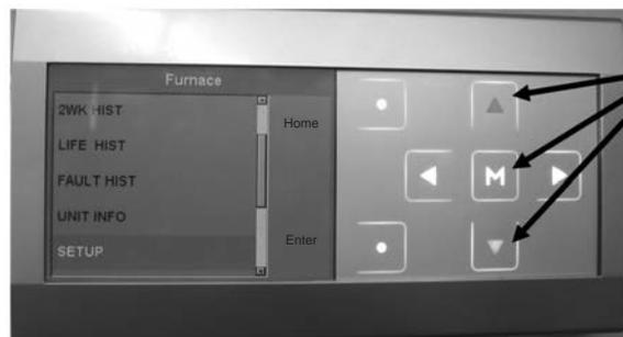
4. The furnace menu options will appear. Use the up and down arrow keys to navigate to the **SETUP** menu. Press "**M**" to enter the menu. Next, the next screen below will appear.
