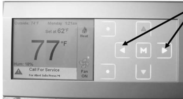
1. From the main screen, press the left and right arrow keys together at the same time for at least 3 seconds. The next screen below will appear. (Note that Call for Service appears at the bottom of the screen. This is an indicator that the fault messages should be viewed to determine the cause of the fault.)
