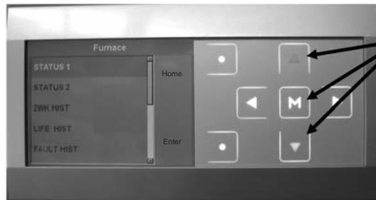
4. The furnace menu options will appear. Use the up and down arrow keys to select the desired menu. Next, press "**M**" to enter the desired menu. Next, the next screen below will appear.
