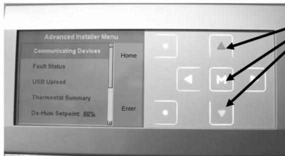
2. The **ADVANCED INSTALLER MENU** is displayed. Use the up and down arrow keys to highlight **Communicating Devices**. Next, press the "**M**" key. The next screen below will appear.
