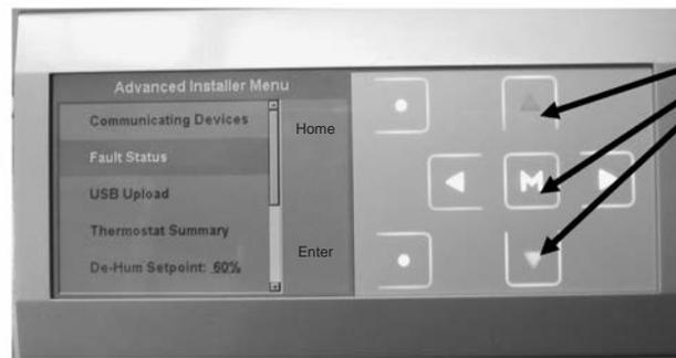
2. The **ADVANCED INSTALLER MENU** is displayed. Use the up and down arrow keys to highlight **Fault Status**. Next, press the "**M**" key. The next screen below will appear
