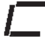
Flashing lower case c A call for first stage cooling has been received
