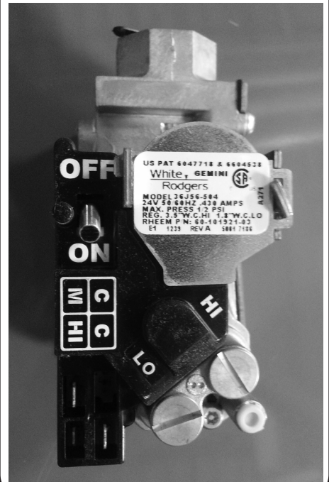
FIGURE 3B WHITE RODGERS 2-STAGE GAS VALVE
