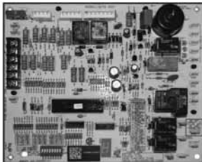
INTEGRATED FURNACE CONTROL
