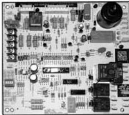
INTEGRATED FURNACE CONTROL
