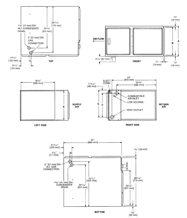
IMPORTANT NOTE: Horizontal furnace may be installed for horizontal left hand air supply ONLY. The condensate trap provided for horizontal application must be installed in the field beneath the unit as directed in the furnace Installation & Operating Instructions.
