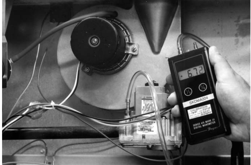
FIGURE 16 TYPICAL HOSE CONNECTION TO LINE PRESSURE TAP
