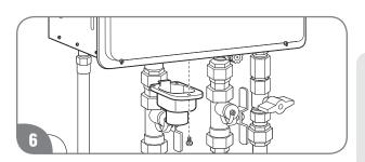
Reinstall the remote control connection cover and secure with the one screw.
