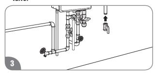
Install a manual gas supply line shut-off valve to the end of the gas supply line.
