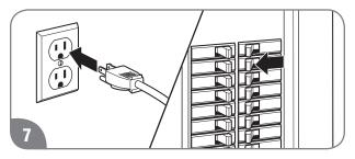
Switch on the power supply to the water heater. Check for proper operation of the remote control and the water heater.
