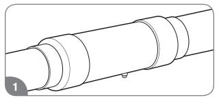
One trap method: Glue a 3" by 4" adapter coupling to each end of a 4" PVC pipe length. Drill a ½" hole in the side of the larger diameter pipe. Tap and thread for a ½" barbed fitting, install fitting. Install the collector with the fitting facing down. DO NOT install in verticial position. Connect a drain hose to the fitting and clamp, run hose to a suitable drain.
