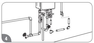
Using the proper-size piping, fittings, and components, build the gas supply line to the water heater.
