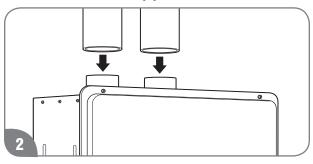
Complete the vent pipe installation to the water heater's vent connector fittings. Use cleaner-primer and PVC appropriate cement where the vent pipes ioin the water heater.
