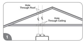
Cut a hole through the roof and interior ceiling to accommodate the vent pipes.
