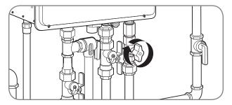
The water heater must be isolated from the gas supply piping system by closing the manual gas shut-off valve during any pressure testing of the gas supply piping system at test pressures equal to or less than 1/2 psi (3.5 kPa).
