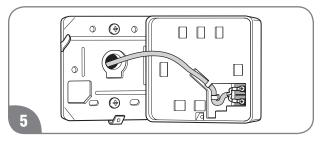
Connect the remote control to the remote control cable.
