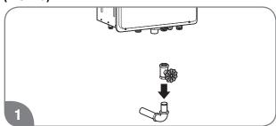
Install a COLD water shut-off valve near the inlet line on the water heater. This valve will be used for servicing and draining purposes.
