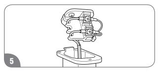
Secure the remote control extension cable on the hook located on the side of the remote control connection base.
