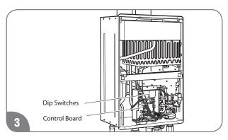
Find DIP Switch 2 located in the top-right portion of the control board. The switch labeled "DIP 2" is the bottom switch.
