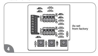
The factory settings for this switch should all be in the OFF position (DOWN).
