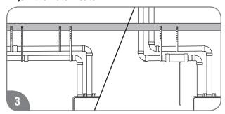
Support vertical and horizontal runs as described on page 35. Vertical supports are required every 4 ft. (1.2 m) along a vertical pipe route, after every transition to vertical, and after every offset elbow.
