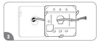
Feed the remote control cable through the large center hole in the base plate.
