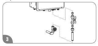
Install a service valve on the end of the COLD water supply line and connect it to the water inlet on the water heater.
