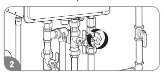
Turn the gas shut-off valve clockwise to the OFF position. This valve is located on the outside of the water heater. Wait 5 minutes to clear any gas. If you don't smell gas, proceed to Step 3.
