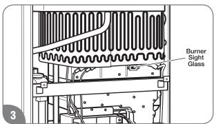
While the water heater is operating, inspect the main burner flames through the burner sight glass. The flames should be blue when the main burner is firing.
