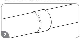
Attach the female end of the next vent pipe section to the male end of the 2-in./3-in. (5.1-cm/7.6-cm) vent pipe. See "Cementing Joints" on page 40.
