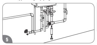
Install a sediment trap at the lowest portion of the gas line.
