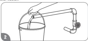
Before attaching the water line to the water heater, open the shut-off valve. Run the water until it has purged all contaminants (sand, debris, air, caulking, etc.).
