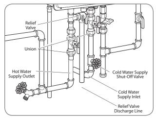
One end of the relief valve discharge line connects to the HOT water outlet pipe as shown above. The other end of the pipe should be routed to a suitable drain to eliminate potential water damage.
