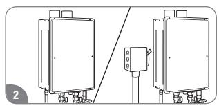
Make sure the proper electrical outlet or supply (120 VAC/60 Hz) is available and located near the unit. Direct-vent models come with a 6-ft. (1.8-m) power cord, while the outdoor models require hardwiring or the addition of a plug.
