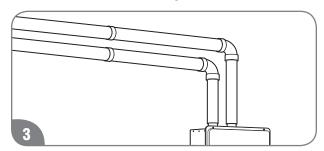
Complete the rest of the vent pipe installation to the water heater's flue outlet and air intake.
