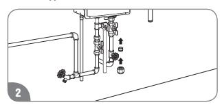
Install a ground joint union or ANSI design-certified semi-rigid or flexible gas appliance connector to the open end of the manual gas appliance shut-off valve. The NFGC, ANSI Z223.1 and CAN/CSA B149.1 codes mandate the use of manual gas shut-off valve.
