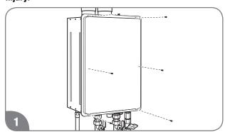
Remove 6 screws and the unit cover panel.
