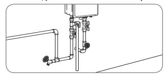
It is recommended to use unions and flexible copper connections at the COLD and HOT water lines. They allow the water heater to be disconnected easily for servicing.
