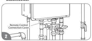
Loosen the one screw located on the remote control connection cover. The connection cover is made of white plastic.
