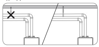
Stress levels in the pipe and fittings can be significantly increased by improper installation. If rigid pipe clamps are used to hold the pipe in place, or if the pipe cannot move freely through a wall penetration, the pipe may be directly stressed, or high thermal stresses may be formed when the pipe heats up and expands. Install accordingly to minimize such stresses.
