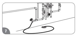
Connect a garden hose to the drain valve in the hot water outlet line and place the other end in a suitable drain. Open the drain valve until all the water has drained from the water heater. Leave water heater as is until placed back in service.
