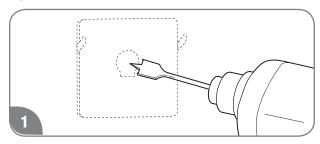
Drill a 1- to 1 1/2-in. (2.5/3.8-cm) hole at the proposed control location. Install the remote control cable between the location of the remote control and the water heater.
