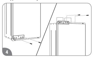
Using two mounting screws and washers, secure the lower mounting bracket to the wall. Then, secure the upper mounting bracket to the wall with two mounting screws and washers.
