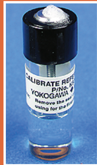
The super sensitivity of the Big Blu fluid is demonstrated by micro-foam “cocooning” of R-11 vapor off a reference leak.
