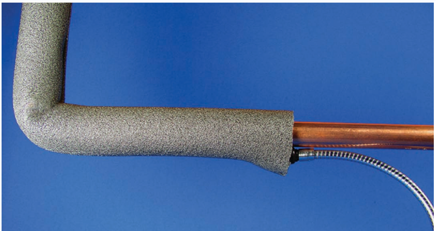
An insulated pipe being scanned for leakage. It is important that the insulating material is not glued to the metal pipe and does not have any open gaps or tears.
