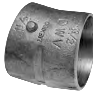
808 \Delta DWV 22 1 / 2 ° Elbow C x C – Cast
