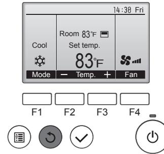
Press the [RETURN] button to exit the Main menu and return to the Main display.
