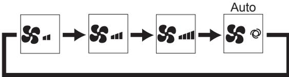
• The available fan speeds depend on the models of connected indoor units.
