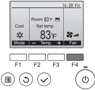
Press the [F4] button to go through the fan speeds in the following order.
