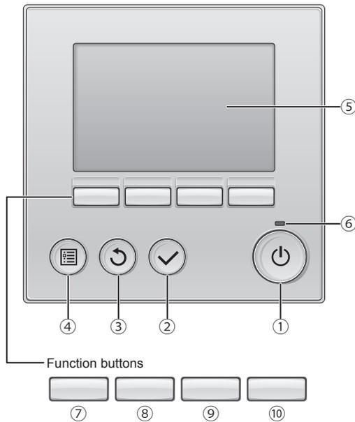
The functions of the function buttons change depending on the screen. Refer to the button function guide that appears at the bottom of the LCD for the functions they serve on a given screen. When the system is centrally controlled, the button function guide that corresponds to the locked button will not appear.
