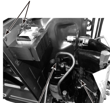
Discharge pipe brazed part
