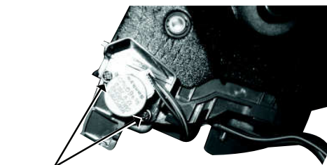
Screws of the damper lock motor (Right)
