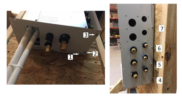
7. Attach enclosure blank side (item #4) to the enclosure using same order as previous step.
