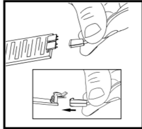
**Note:** The Water Leak Sensor comes with a paper sleeve. The paper sleeve acts as a barrier between the Leak Sensor and metal. If the Leak Sensor makes contact with metal, it will signal the LeakSmart Valve to shut-off. When the paper sleeve becomes wet, it will signal the LeakSmart Valve to shut-off. Make sure the paper sleeve is completely dry when using it with the Leak Sensor. If the Leak Sensor will not be contacting metal, you may remove the paper sleeve.
