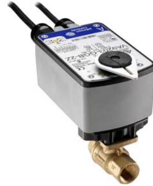
VG1000 Series Two-Way, Spring Return, Stainless Steel Ball and Stem Ball Valve Assemblies with End Switches
