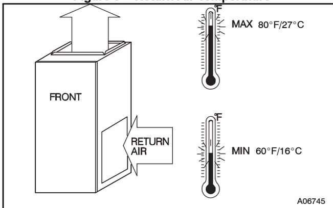
This furnace is designed for minimum continuous return-air temperature of 60°F (15°C) db or intermittent operation down to 55°F (13°C)db such as when used with a night setback thermostat. Return-air temperature must not exceed 80°F (27°C) db. Failure to follow these return-air temperature limits may affect reliability of heat exchangers, motors, and controls. (See Figure 3)
