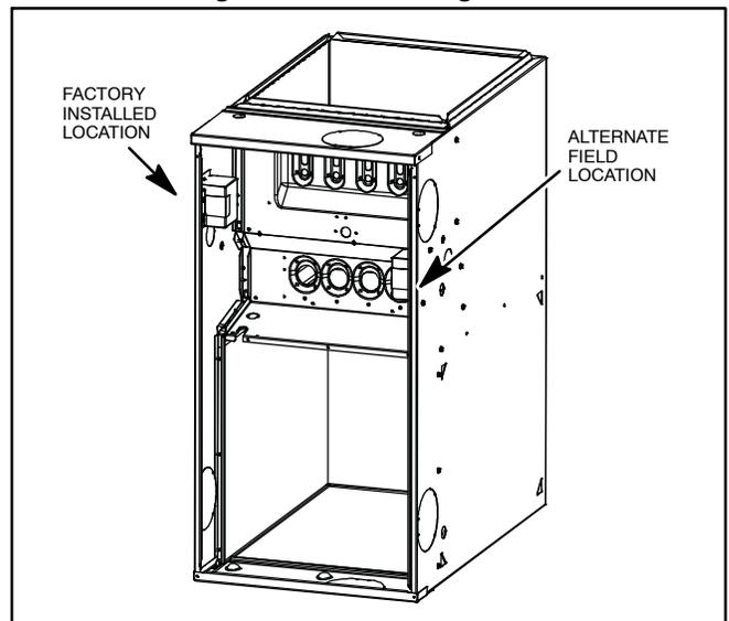
4. Remove and save two screws holding J-Box. (See **Figure 23**)
