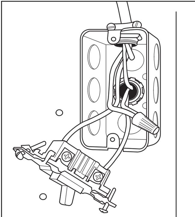
12. Complete electrical box wiring and installation. Connect line voltage leads as shown in **Figure 24**. Use best practices (NEC in U.S. for wire bushings, strain relief, etc).
