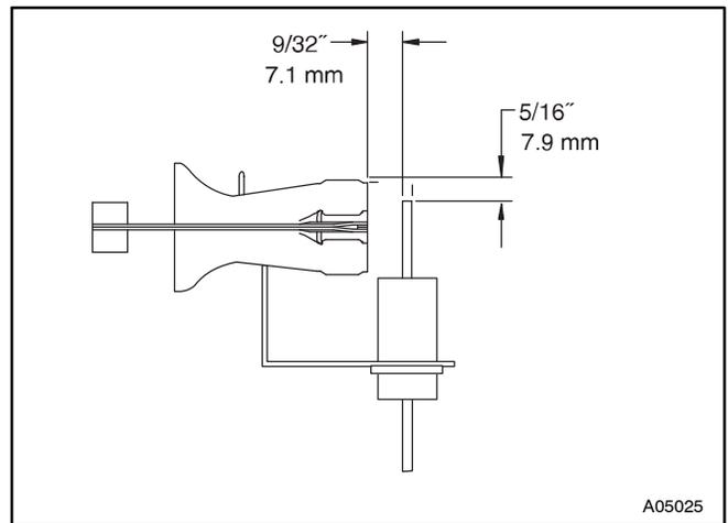
**Figure 53 – Igniter Position – Top View**
