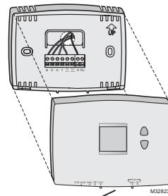
Pull at bottom to remove thermostat from wallplate.
