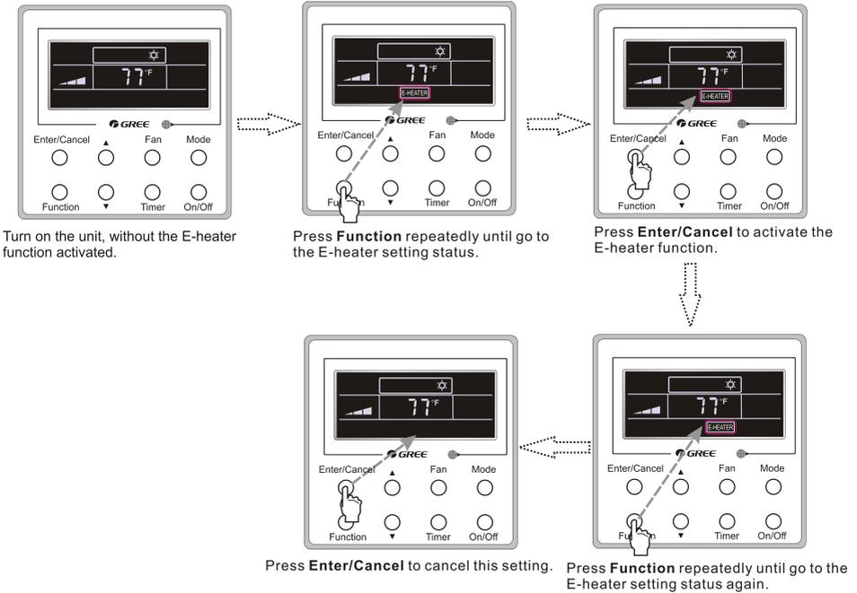
Fig.3.9.1 E-heater Setting
