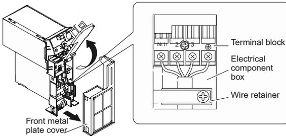
3. Secure interconnecting wires to the terminal block as shown in the connection diagram above.
