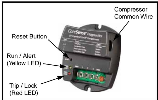
**Figure 2. CoreSense™ Diagnostics Module**
