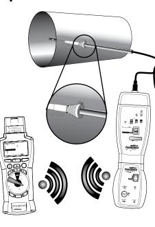
RCONE1 and AAT3 working with ET2W and HG3 to wirelessly log Wetbulb for target superheat testing.
