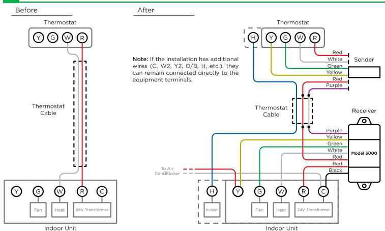
B Adding an Air Conditioner to a Heat-Only System (Dry-Contact Switching)
