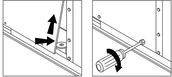
Fig. 10 — Replacing the Gas Component Access Panel
