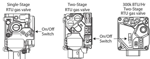
**Fig. 18 — Single and Two-Stage Gas Valves**
