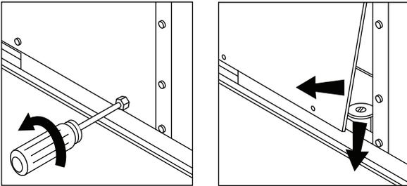
Fig. 8 — Gas Component Access Panel Removal
