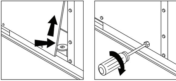
**Fig. 19 — Replacing the Gas Component Access Panel**
