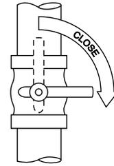
**Fig. 15 — Gas Supply Shut Off Valve**
