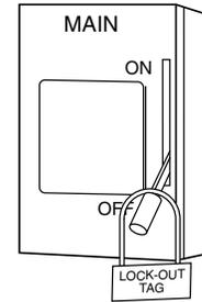
**Fig. 16 — RTU Main Disconnect — Electrical Supply**
