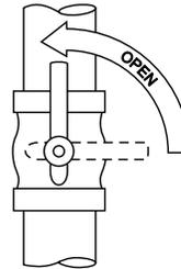
Fig. 12 — Gas Supply Shut Off Valve
