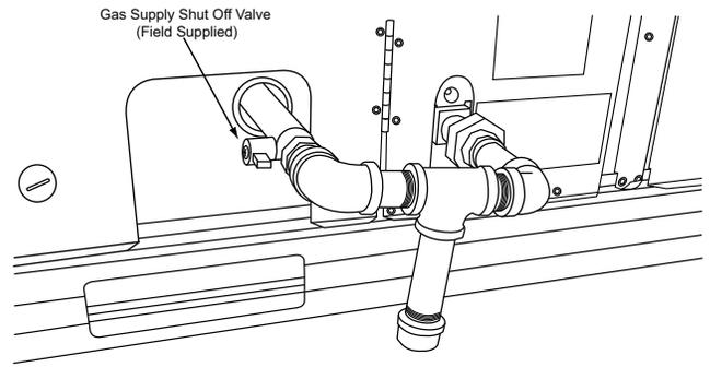
**Fig. 2 — Gas Supply Shut-Off Valve Location — 3 to 12<sup>1</sup>/<sub>2</sub> Ton Units (Thru-the-base gas supply shown)**
