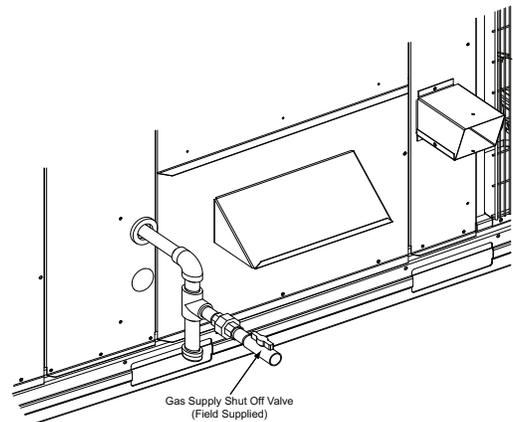
**Fig. 3 — Gas Supply Shut-Off Valve Location — 15 to 27<sup>1</sup>/<sub>2</sub> Ton Units**
