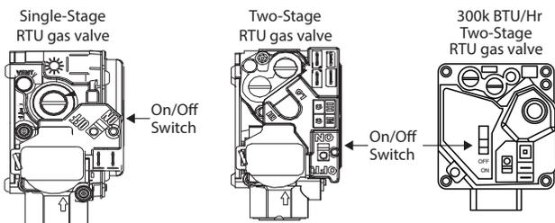
Fig. 9 — Single and Two-Stage RTU Gas Valves
