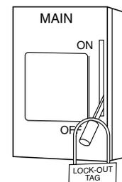
**Fig. 5 — RTU Main Disconnect — Electrical Supply**
