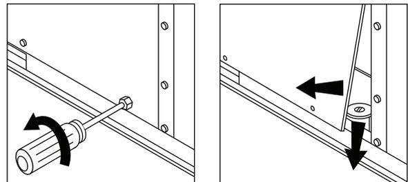
**Fig. 17 — Gas Component Access Panel Removal**
