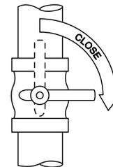
**Fig. 4 — Gas Supply Shut Off Valve**
