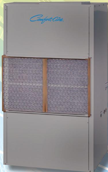
These individual packaged units transfer heat via water loop systems for effective heating and cooling. Our largest capacity units, they feature belt drive blowers and reliable scroll compressors. Power and water connections can be made on either side (also refrigerant connections for HKV), and discharge air is field convertible.
