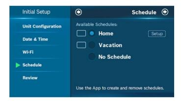
**HOME:** You can use this schedule to set your heating/ cooling equipment to predefined set points. The device initially comes with a factory default schedule, which can be adjusted as necessary.
