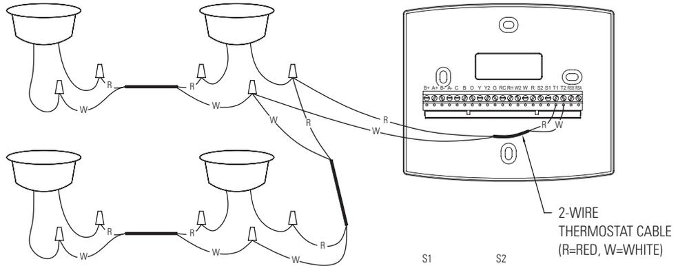
**FOUR SENSOR TEMPERATURE AVERAGING – WIRING**
