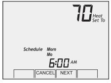
Continuing pressing the **NEXT** key to display the morning, day, evening and night schedule along with the heating and cooling temperatures for each day of the week. Press the **CANCEL** key at any time to exit and return the thermostat to normal operation.
