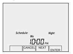
Mo (Monday) will appear on the LCD. Continue to press the **NEXT** key to add additional days of the week. Use the **Up** and **Down** keys to turn days ON or OFF. The schedule will be applied to the days that are ON. These days will be displayed on the thermostat. The example below shows a schedule being applied to Monday through Friday.
