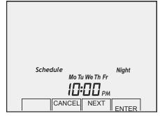
Pressing the **ENTER** key will copy and save the schedule for the days of the week selected. After the **ENTER** key is pressed, the thermostat will return to normal operation To change the schedule for other days of the week, repeat the same programming steps.
