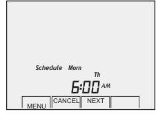
Press the **NEXT** key to display the morning heating (**Heat**) temperature. Use the **Up** or **Down** keys to change the temperature.
