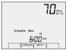
Press the **NEXT** key to display the morning Cooling (**Cool**) temperature. Use the **Up** or **Down** keys to change the temperature.
