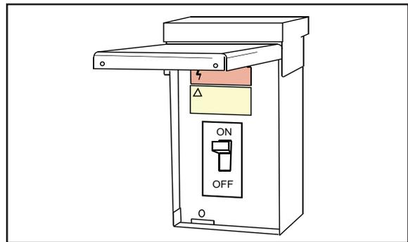
**STEP 4** - Wait one (1) hour before starting the unit if compressor crankcase heater accessory is used and the Outdoor Ambient is below 70°F.
