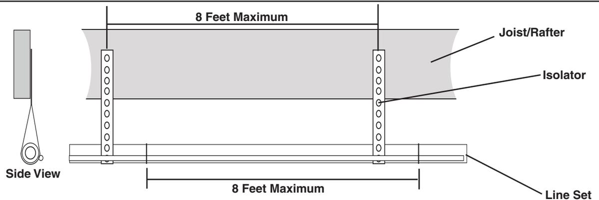
Secure Vapor line from joists using isolators every 8 ft. Secure Liquid Line directly to Vapor line using tape, wire, or other appropriate method every 8 ft.
