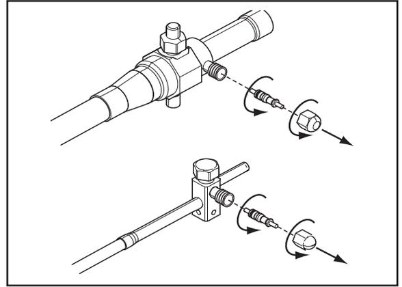
**STEP 3** - Purge the refrigerant lines and indoor coil with dry nitrogen.
