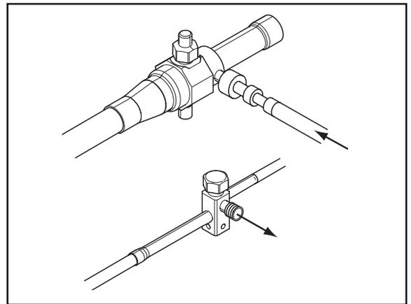
**STEP 4** - Wrap a wet rag around the valve body to avoid heat damage and continue the dry nitrogen purge.
