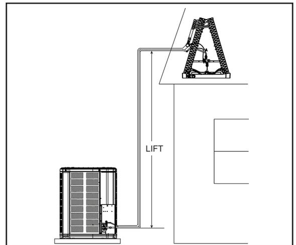
**STEP 2** - Determine the final subcooling value using total Line Length and Lift measured in STEP 1 and the charts below.
