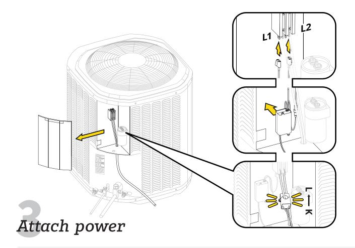
NOTE: CLASS 2 WIRING TO BE ROUTED SUCH THAT IT WILL NOT COME INTO CONTACT WITH LINE VOLTAGE WIRING
