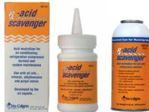
An effective way to neutralize or "scavenge" acid in refrigeration and air conditioning systems. Use after burnouts or during normal on-going system maintenance. Normal dosage rate is 2 fluid ounces for every one gallon of system oil. For use with all common refrigerants and oils (mineral, alkylbenzene and POE).
