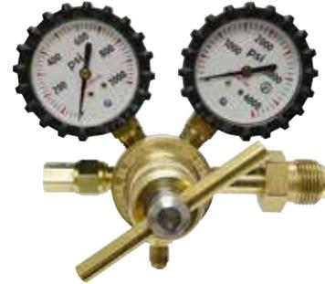
Nitrogen Regulator with a Delivery Pressure 0-800 PSI for purging and pressure testing air conditioning and refrigeration systems. A durable brass piston designed diaphragm regulator with CGA580 inlet connection, 1/4 inch male flare outlet connection, self re-seating relief valve (not designed to protect downstream system) and easy to read 2 inch Contents Gauge 0-4000 PSI and Delivery Gauge 0-1000 PSI with protective rubber gauge boots.
