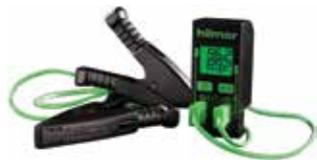
Makes Calculations Easier: The industry's only manifold-compatible compact thermometer with two readings to help simplify the calculation of superheat and subcool. Superior Versatility: Use it on any gauge set, or remove it and use it independently. Reads Temperatures Quickly: Two easy-to-use, K-style tube clamp thermocouples get you to the temperature reading quickly.
