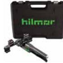
Simple Setup: Universal crossbar and color-coded mandrels make identifying and changing sizes quick and easy. One-handed Operation: A ratcheting mechanism and innovative release lever allow for bending with one hand. Small Space Capable: A compact design allows it fit where others can't. Quality Finish: An advanced mandrel design reduces frustration and makes it simple to release the tube.
