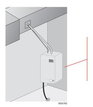
Remote mounting. The Electrode Steam is installed some distance away from your furnace supply duct. An insulated hose carries steam from the Electrode Steam to a suitable location on the supply duct.
