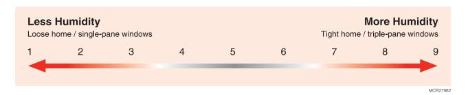
Manual humidity controls do not have built-in frost settings. They require you to adjust the humidity setpoint when the outdoor temperature changes. Use higher humidity setpoints when the temperature is warmer, and lower setpoints when the temperature is cooler.
