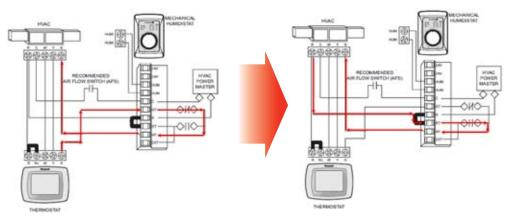
• TrueSTEAM sends this signal when water temperature in the tank is at 170°F (just before boil). This ensures room temperature air isn't
