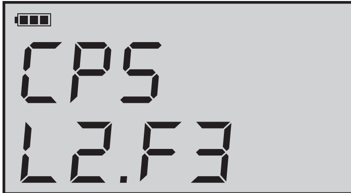
Figure - 1: Displays the software version of the unit.
