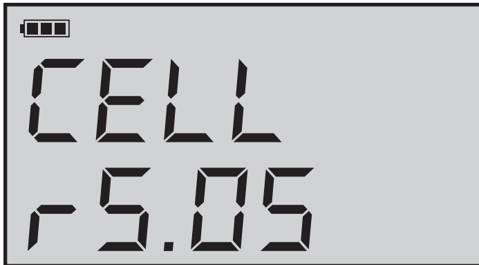
Figure - 7: Scale platform battery voltage.
