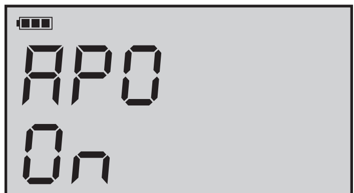
Figure - 6: Scale platform Automatic Power Off status.
