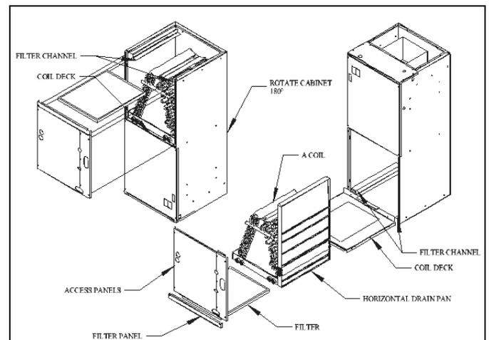
Fig.8. Air Handler parts and changes for Counter flow
