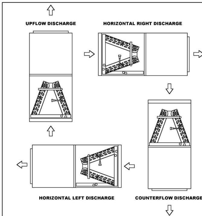
Fig.6. Various airflow orientation
