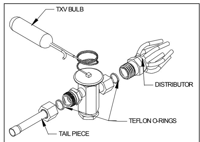
Fig.5. Components of a typical TXV assembly
