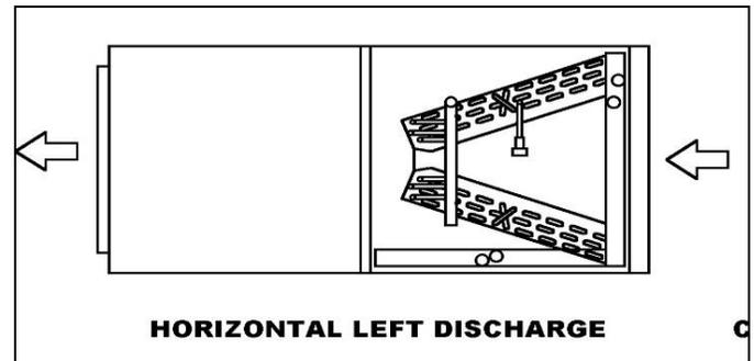
Fig.7. Air flow direction in Horizontal Left application
