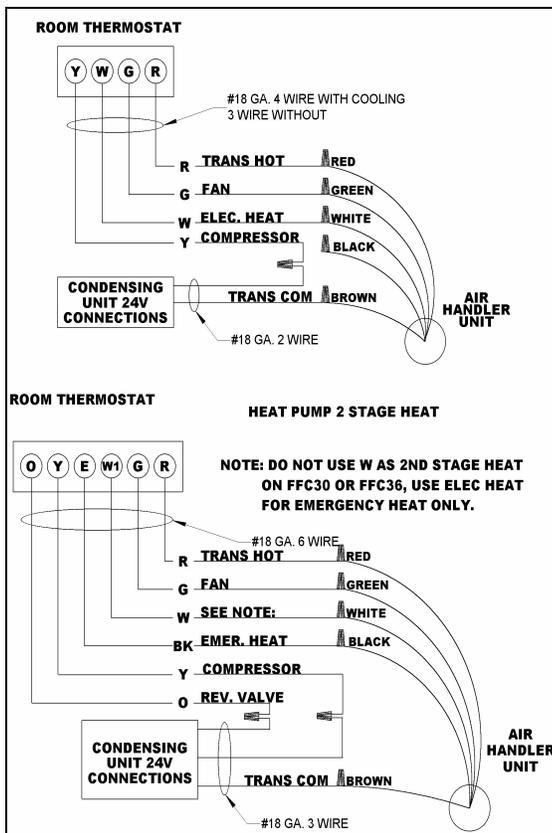
Fig 10. Electric connections
