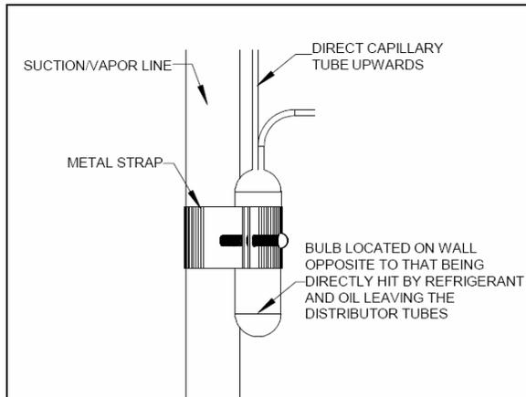
Fig.4. TXV bulb mounted in a vertical orientation
